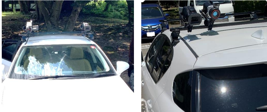
Figure 5 Thermal and HD camera set up
